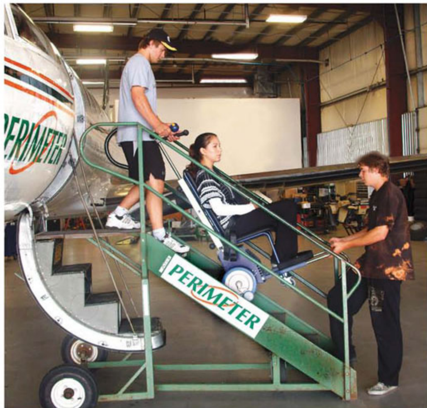
The Amazon Stair Climber weighs only 75 pounds [34 kilograms], yet it can raise or lower a 350-pound [159-kilogram] man up 15 to 20 aircraft stairs. TOP: A medevac flight over Whale Cove, Nunavut.
